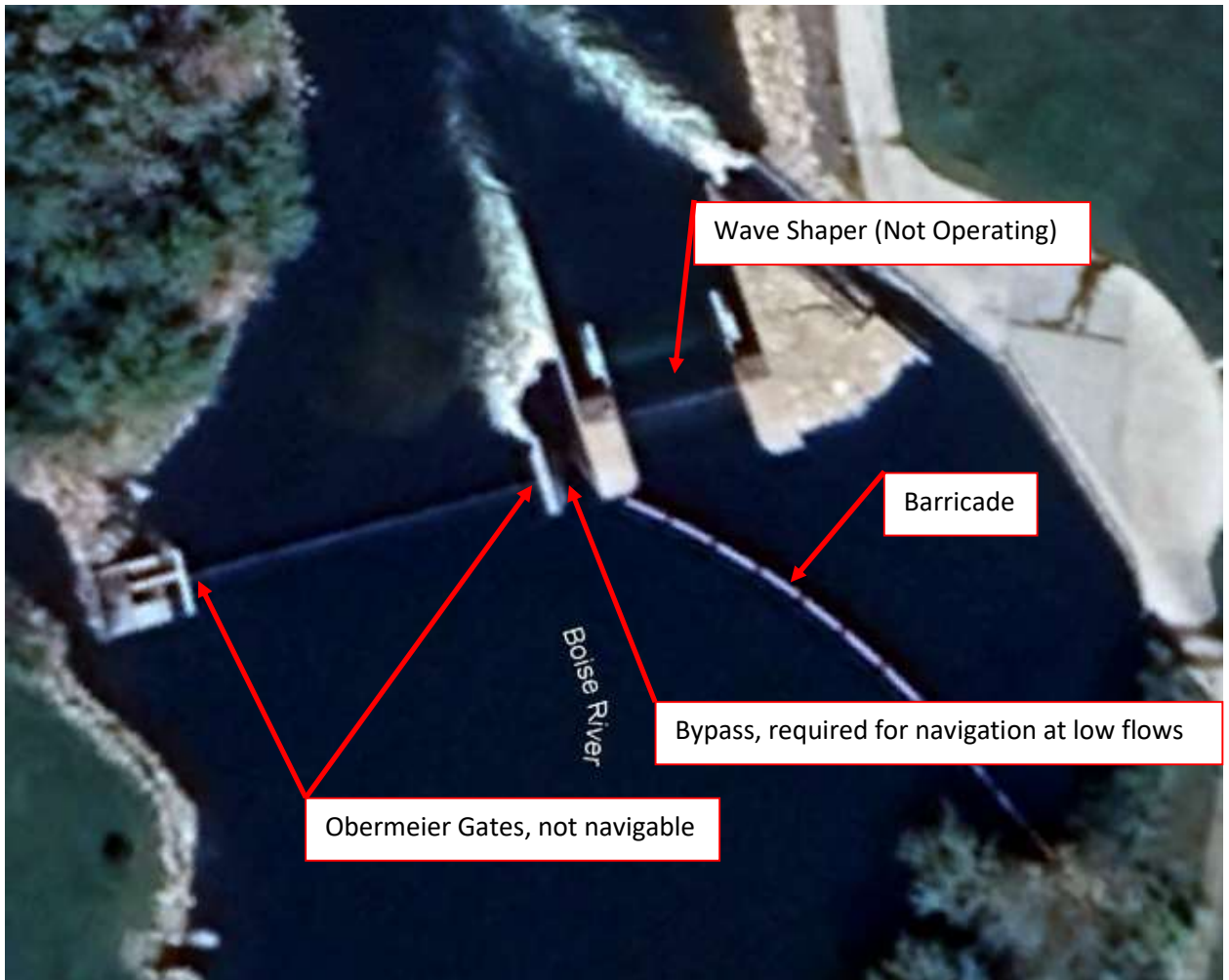
Figure 1. Whitewater Park Phase 2, first feature components at low water, wave shaper not operating.
