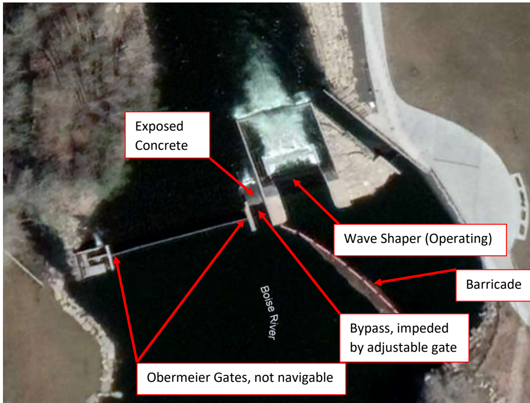
Figure 2. Whitewater Park Phase 2, first feature components at low water, wave shaper operating.
